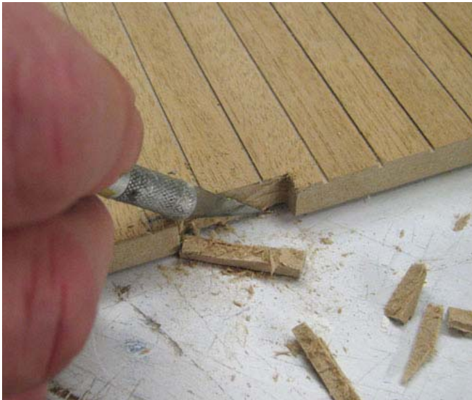
Cutting an Electrification Slot before building
